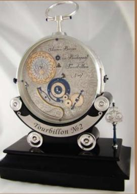
LEFT TO RIGHT FROM ABOVE: The bi-metallic thermometer strip is a purely mechanical way of sensing the temperature; Tourbillon No.2, with a spring Detent Escapement, perpetual calendar, world time, thermometer, and moon phases; The tiny Zappler is about the size of a one of the FDMN watches.
