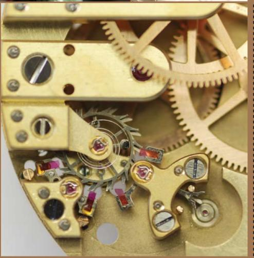
very large size of their balance was chosen on 17 August, the balance diameter was set at 17.08mm. rest of the movement can be designed with this primary element as a kingpin. Each of the two designs had a unique feature; the first being a rather traditional tourbillon. With the
