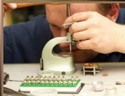
CLOCKWISE FROM TOP LEFT: All the work at the Fabrication de Montres Normandes is done with manually-controlled machines; Carriages 1 and 2 out of three wait their turn to be installed; Karsten Fraessdorf riveting a wheel; Prototype of a new version of the FDMN Constant Force Device; Reaming a hole to the precise size required for jewellery.
