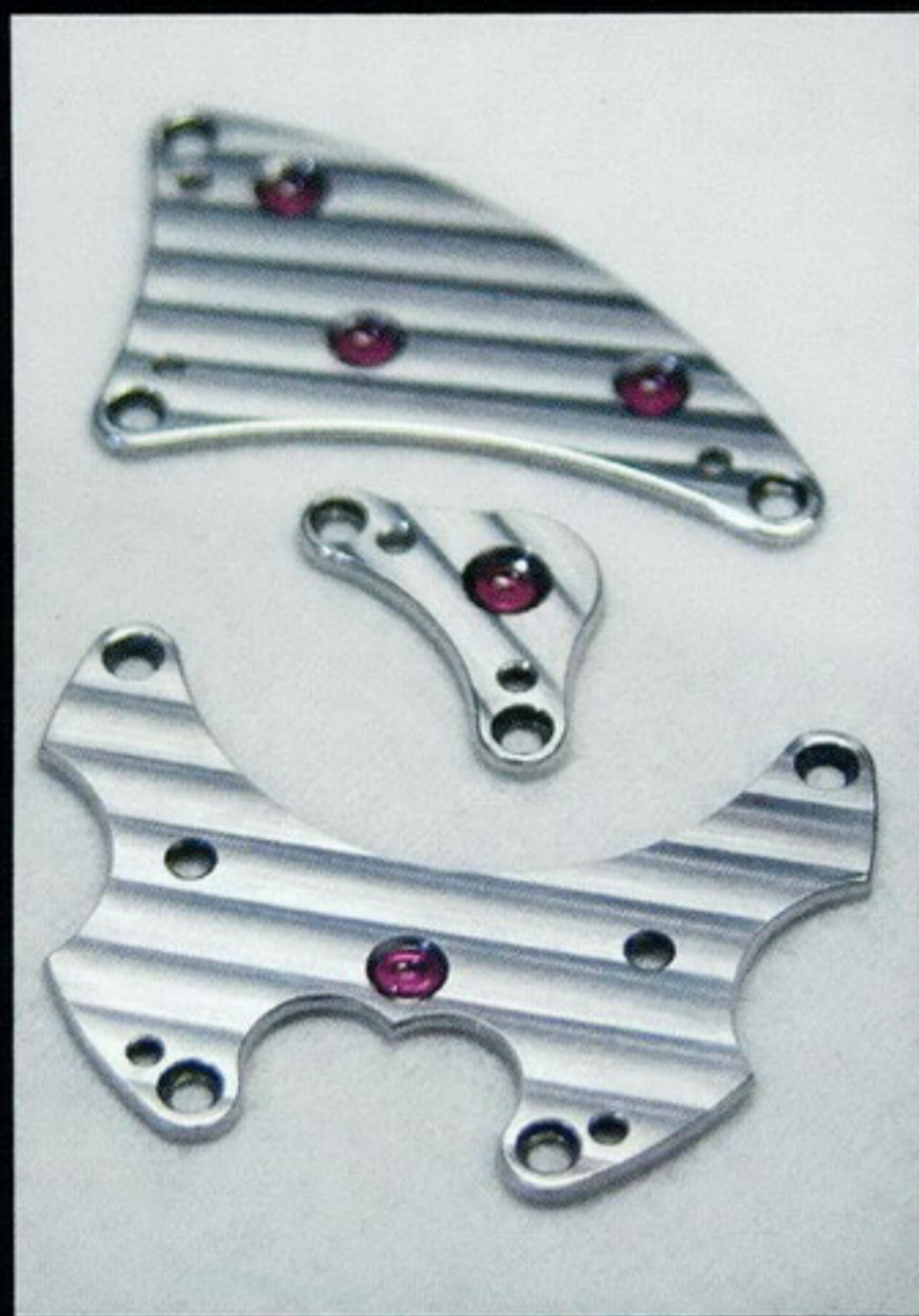
Right: The Primus's 38 x 46 x 17.9 mm case possesses a sapphire crystal window on the side of the tourbillon so that the beauty of this whirlwind can be admired from three sides. Left: The Primus utilizes no ball bearings. It uses synthetic ruby jewel bearings as a traditional movement would.
