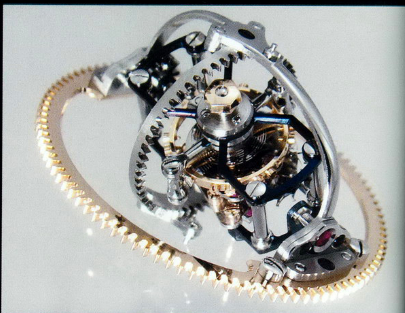
The inner carriage of the Primus triple-axis tourbillon makes one revolution every thirty seconds, the middle one every two and a half minutes, and the outer cage every twelve and a half minutes.
