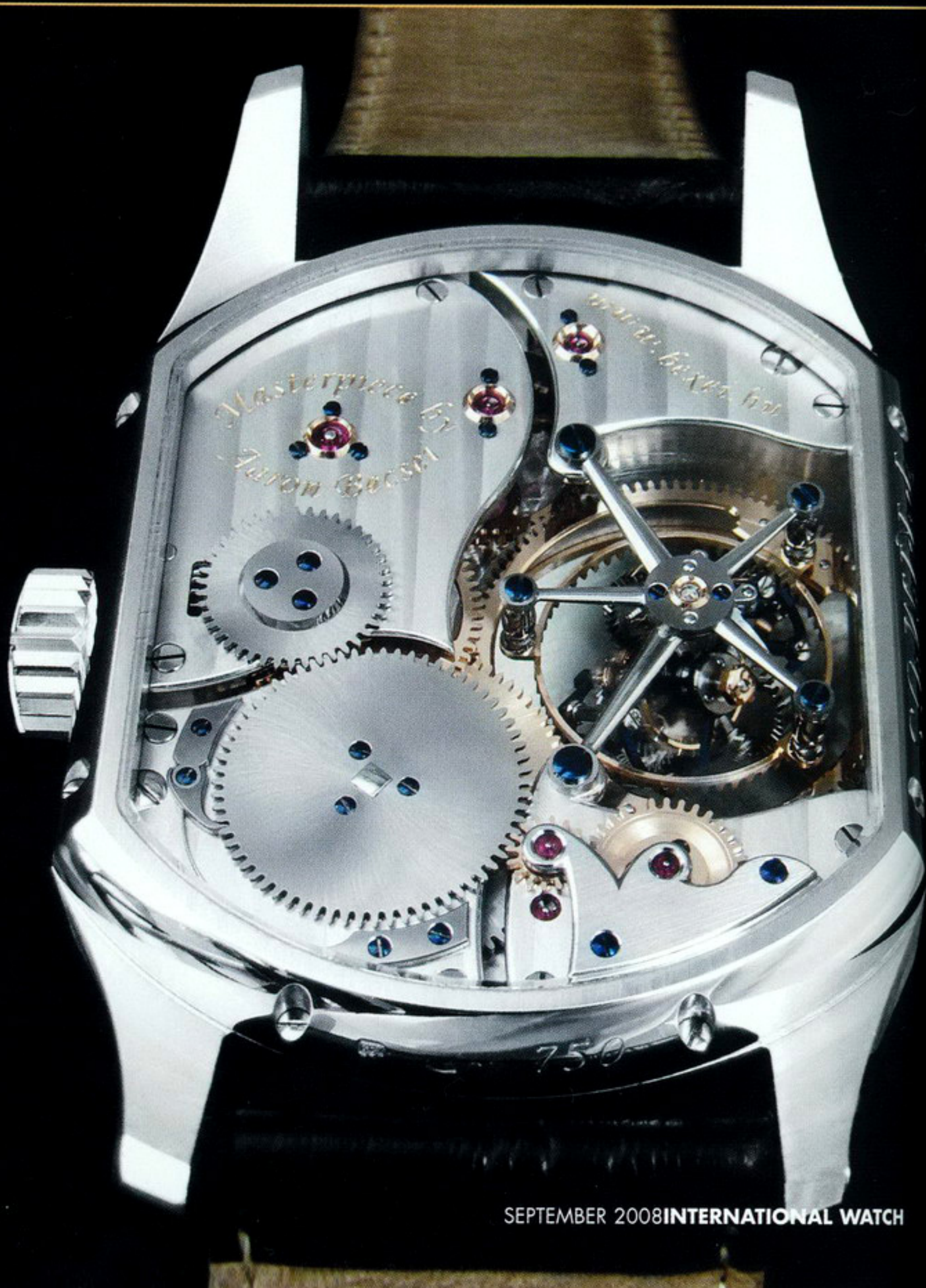
The inner carriage of the Primus triple-axis tourbillon makes one revolution every thirty seconds, the middle one every two and a half minutes, and the outer cage every twelve and a half minutes.
