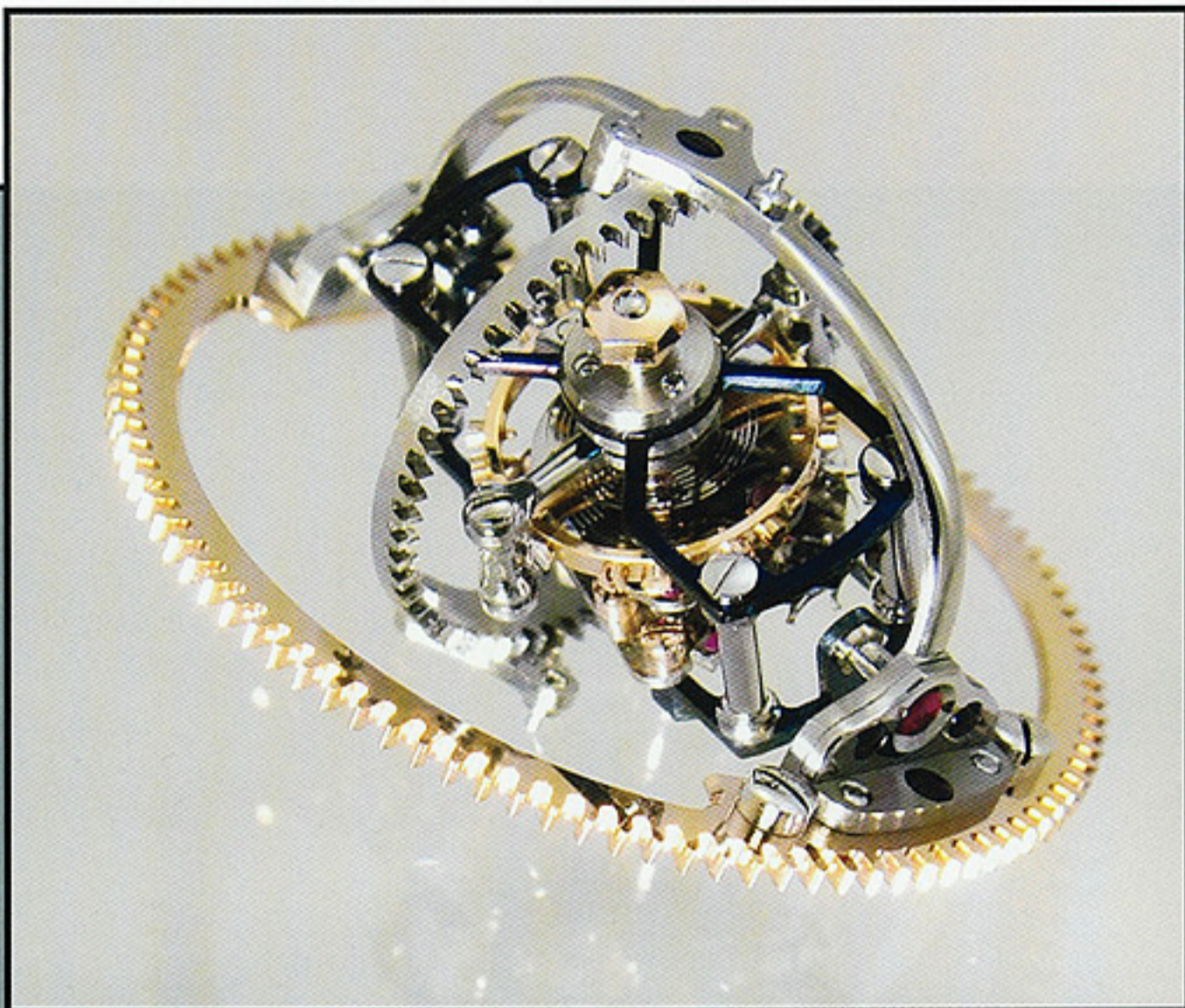
The Primus is a triple axial tourbillon with jewel bearings. The watch shows hours, minutes, seconds and power reserve.
