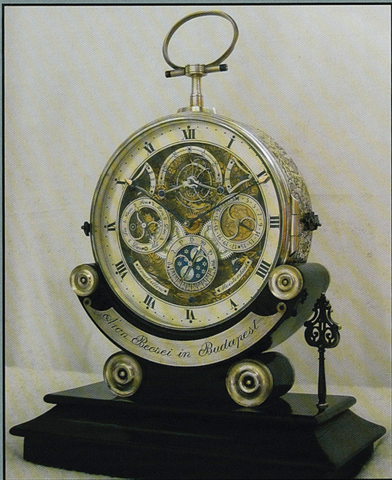
Tourbillon No. 1 features a duplex tourbillon escapement, calendar, moon phase, wind up indicator, world time function and a thermometer. It has a silver case and silver dial, with gold plated wheels and plates.
