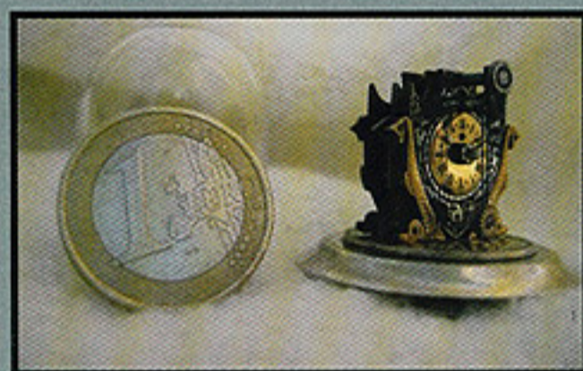
The Miniature Zappler is a double pendulum clock that measures 35 mm tall with its glass dome. It uses a rolling escapement, jewel wheel system and has blued steel hands with silver tips.
